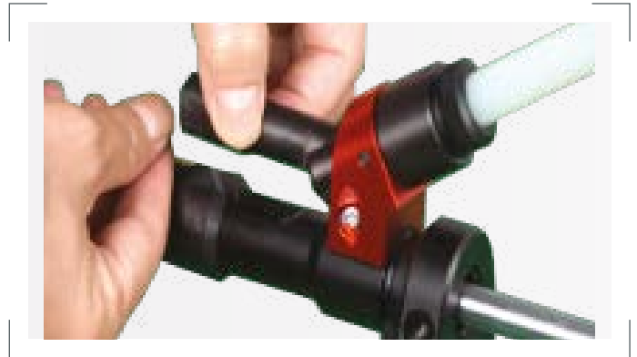
Lift the "swivel" arm to clear screw jam
