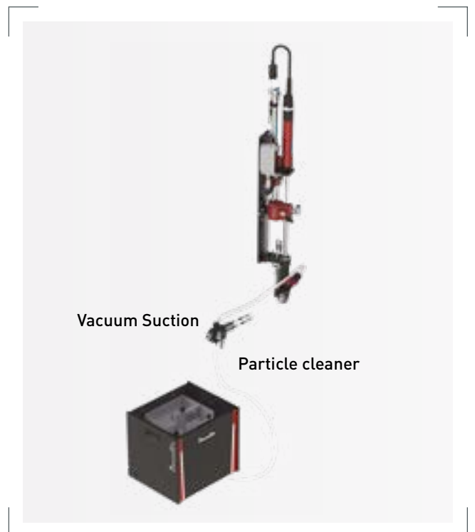
PARTICLE CLEANING in process
