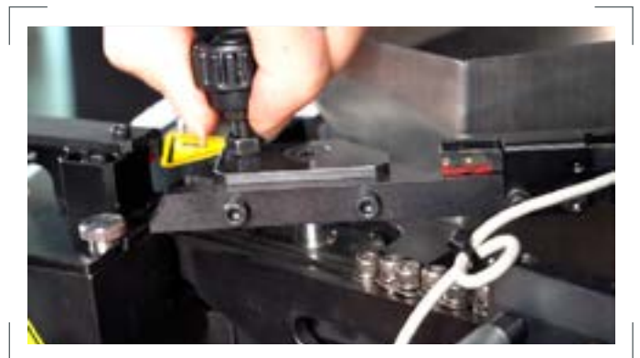
Turn the knob and uplift the upper part of rail
